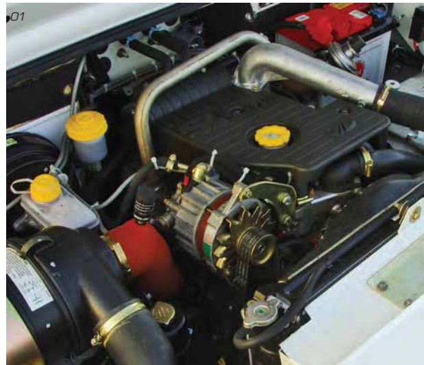
01 The Bolero's 2.5l NEF turbo diesel delivers 74 kW of power and 238 Nm of torque, pulling cleanly from 1800 rpm in third gear, providing great efficiency and excellent fuel economy across any terrain.
